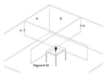
Rotate the laser clockwise so that the forward laser beam passes through mark b1 on wall B. Verify that the plumb dot is on mark x. 10) Mark point **c1** on wall **C**, in the middle of the side vertical beam. (see figure #11).
