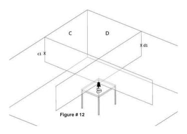
13) Rotate the laser clockwise so that the forward laser beam passes through mark d1 on wall D. Verify that the plumb dot is on mark x. 14) Mark point **a2** on wall **A**, in the middle of the side vertical beam, near point **a1** and at the same height.
