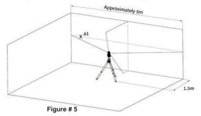
4) Turn the laser level counterclockwise until the right edge of the horizontal beam reaches near **a1**, mark a point **a2** on the wall in the middle of the horizontal beam (see figure 6).
