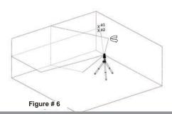
5) The distance between a1 and a2, should be no more than 1 mm, otherwise send the laser level to a qualified technician for repair.
