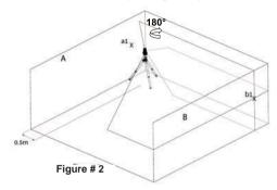
6) Move the laser level towards wall B positioning it at approximately 0.5 meters from wall B and adjust the laser so that the vertical beam passes through point b1.
