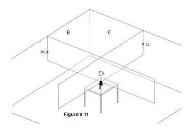
11) Rotate the laser clockwise so that the forward laser beam passes through mark **c1** on wall **C**. Verify that the plumb dot is on mark **x**.
